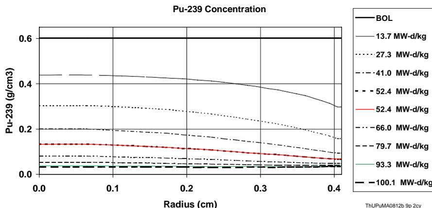
Figure 3 Pu-239 Concentration in center pin during irradiation
