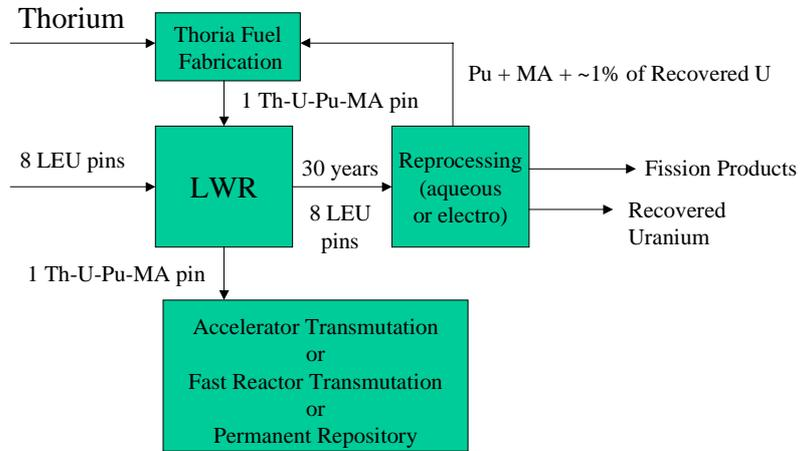
Figure 1 Mono-recycling strategy for Light Water Reactors
