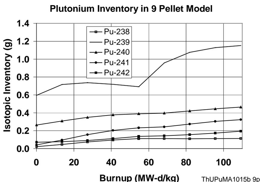
Figure 6 Overall Plutonium Inventory in the 9 Pellet Model
