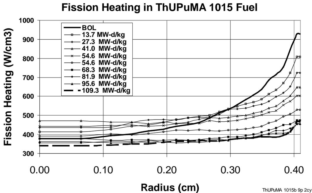
Figure 7 Fission Heating Profile in Transmuter Pellet
