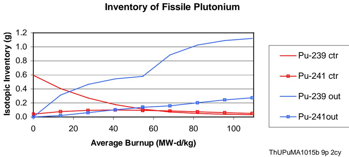
Figure 5 Inventory of Fissile Plutonium Isotopes in the Nine Pellet Model
