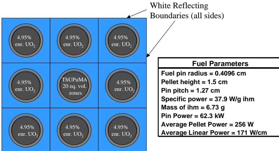
Figure 2 Nine-pellet model and fuel parameters
