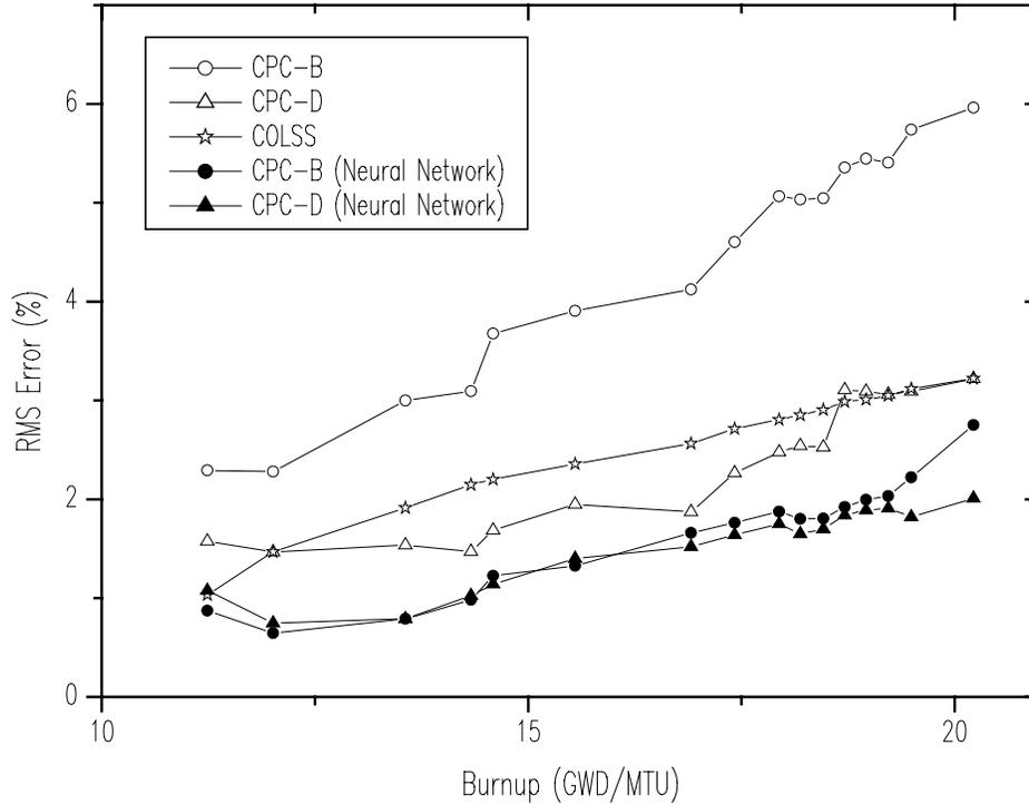
Fig. 5 Comparison between neural networks and protection system signals for YGN-3 cycle 2
