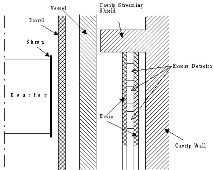
Fig. 1 Radial (4-channel ) and vertical (3-segment ) view of the excor detector system of KSNPs
