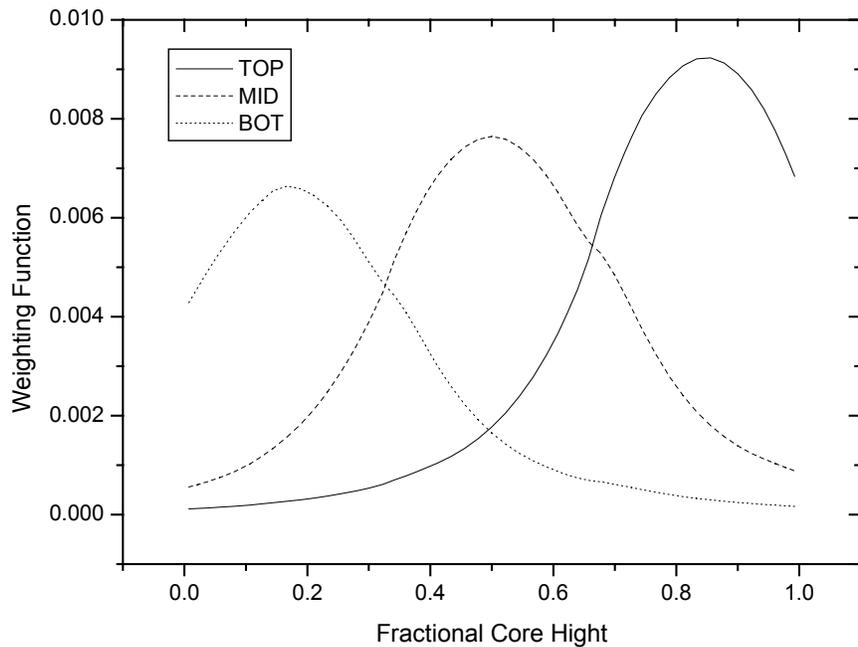
Fig. 3 Axial weighting functions for excore detectors at full power (YGN-3 cycle 1, 500 ppm soluble boron)
