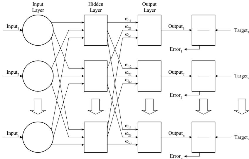
Fig. 2 Typical two-layer feedforward neural network
