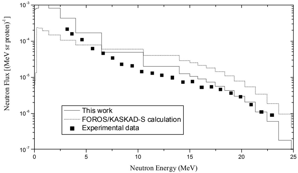
Fig. 3. Energy spectra of neutrons for the copper target bombarded by 30 MeV protons at 0° emission angle.
