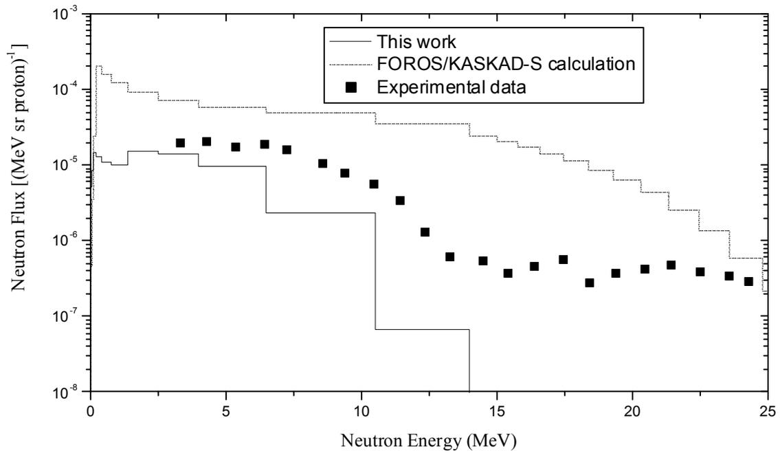
Fig. 1. Energy spectra of neutrons for the carbon target bombarded by 30 MeV protons at 0° emission angle.
