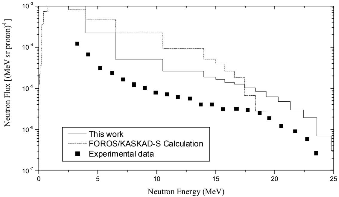
Fig. 4. Energy spectra of neutrons for the lead target bombarded by 30 MeV protons at 0° emission angle.
