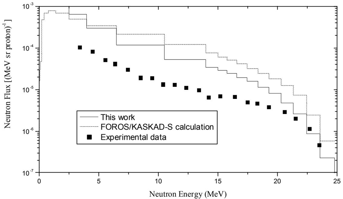
Fig. 2. Energy spectra of neutrons for the iron target bombarded by 30 MeV protons at 0° emission angle.
