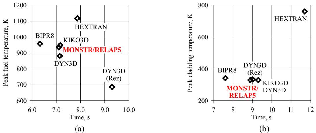
Figure 8. Values and time moments of peak fuel temperature (a) and peak clad temperature (b) in AER-4 benchmark predicted by different codes
