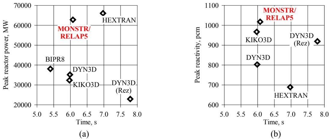
Figure 5. Values and time moments of peak reactor neutron power (a) and peak reactivity (b) in AER-4 benchmark predicted by different codes
