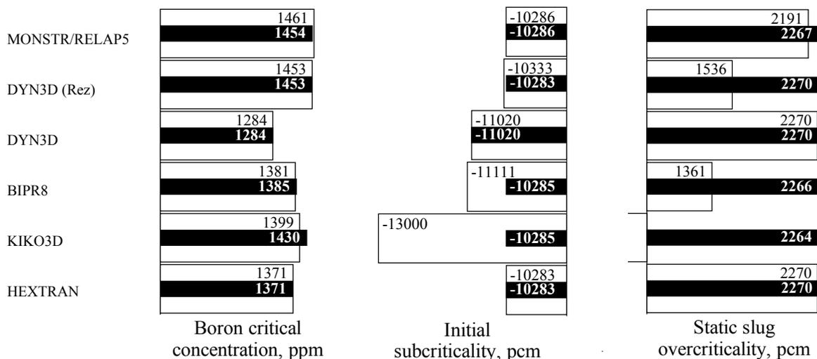
Figure 2. Some key reactivity parameters in AER-4 benchmark calculated by different codes before tuning (white bars) and after tuning (black bars)
