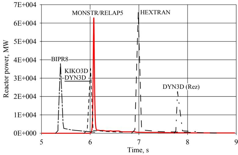
Figure 3. Time history of reactor neutron power in AER-4 benchmark predicted by different codes
