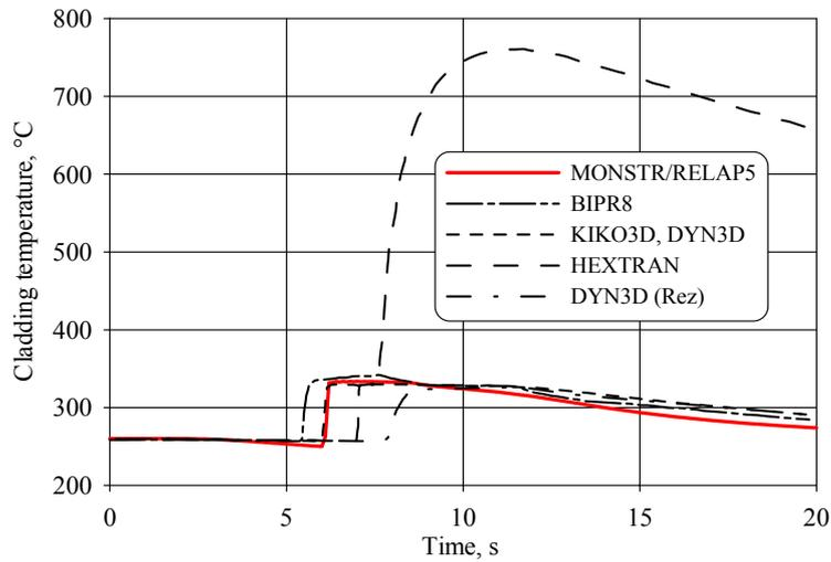
Figure 7. Time history of peak clad temperature in AER-4 benchmark predicted by different codes
