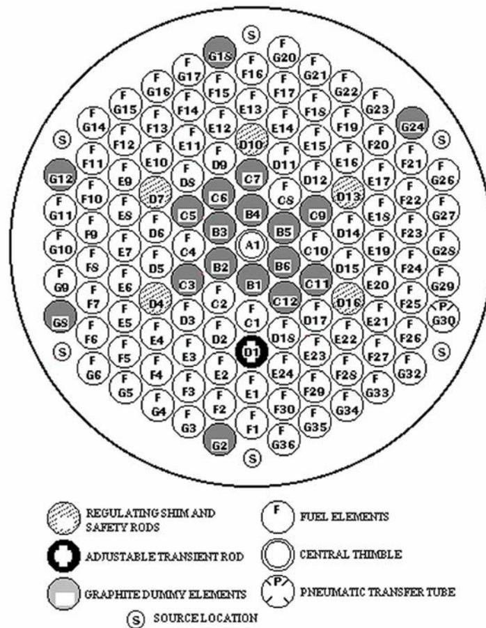
Fig. 2. Final core arrangement of the TRIGA reactor.
