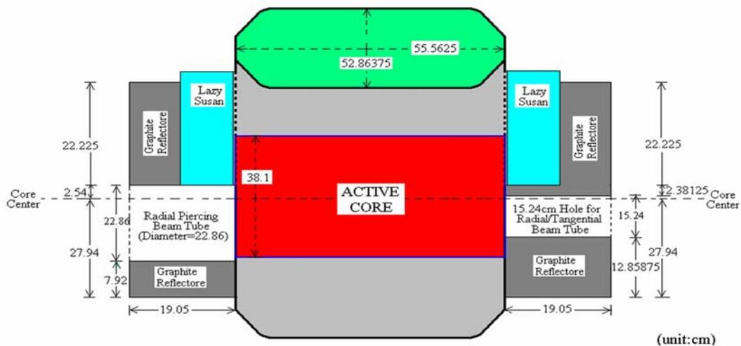
Fig.6. Cutaway view of TRIGA active core including rotary specimen rack Lazy Susan and beam ports.
