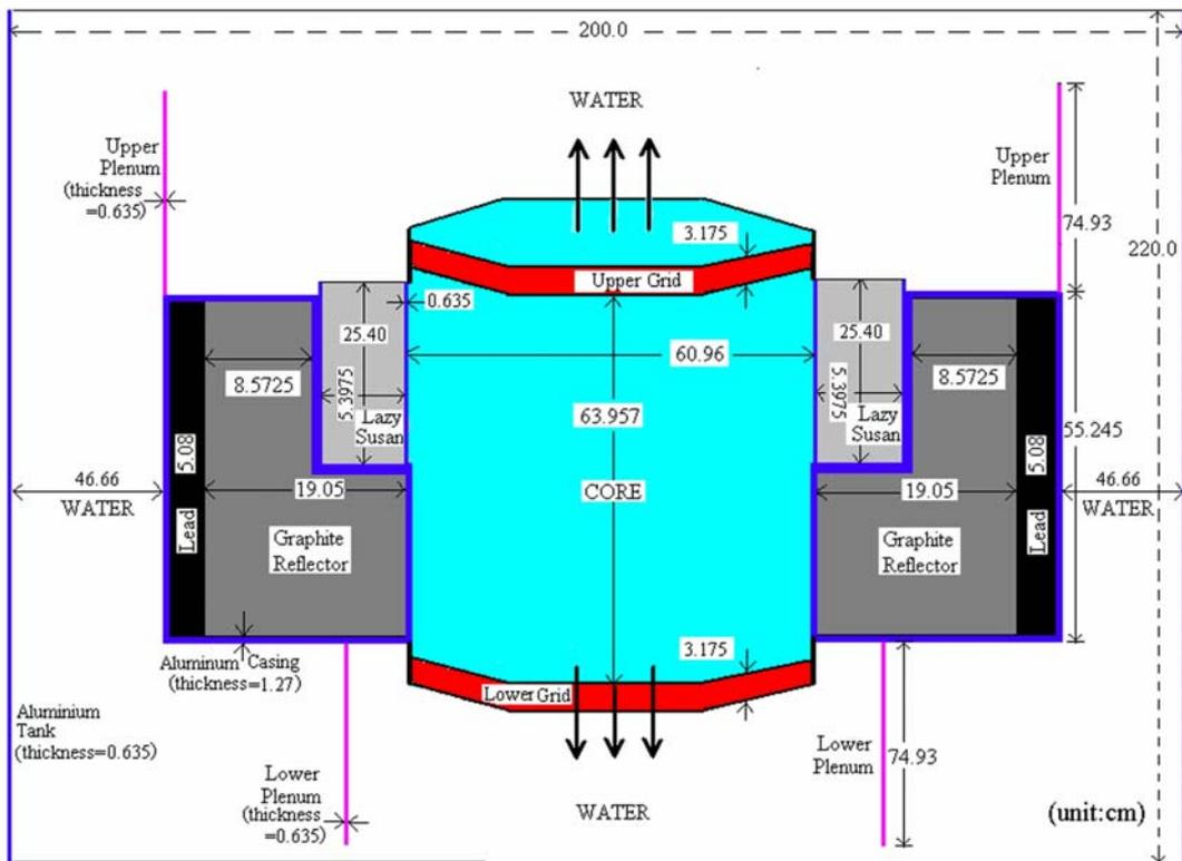
Fig.5. MCNP modeling of TRIGA MARK II research reactor.
