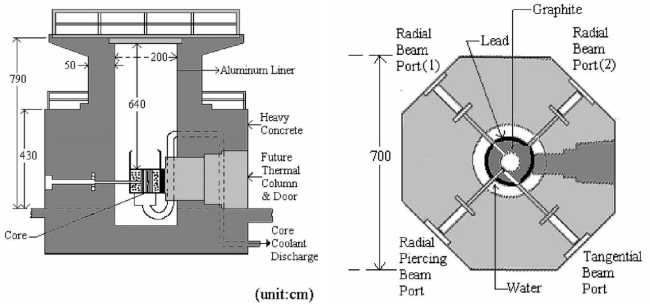
Fig. 1. Cutaway view of TRIGA reactor.
