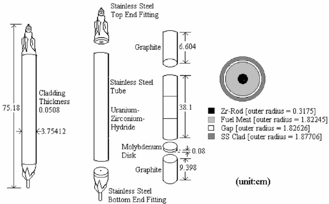
Fig.3. TRIGA stainless-steel-clad fuel element with triflute and fittings.
