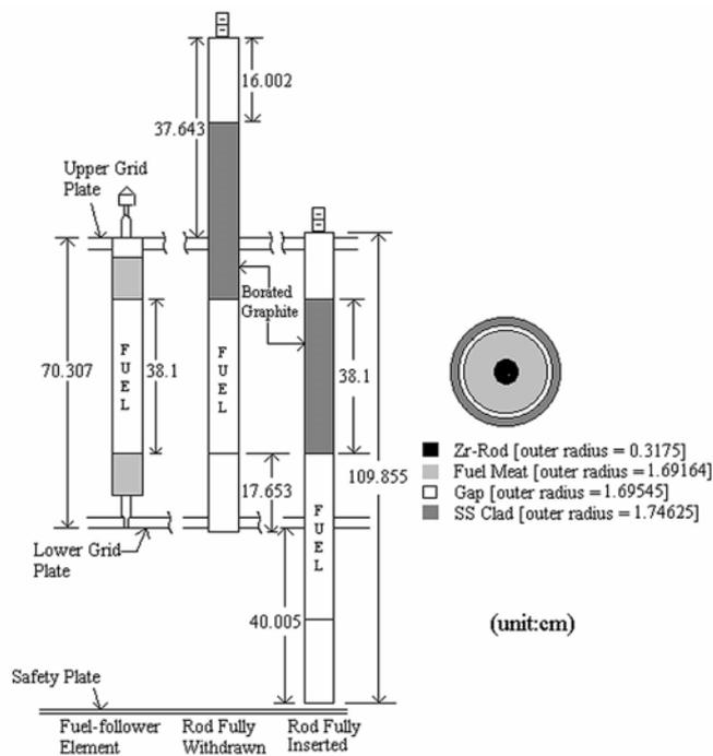
Fig.4. Fuel-follower control rod - withdrawn and inserted position.
