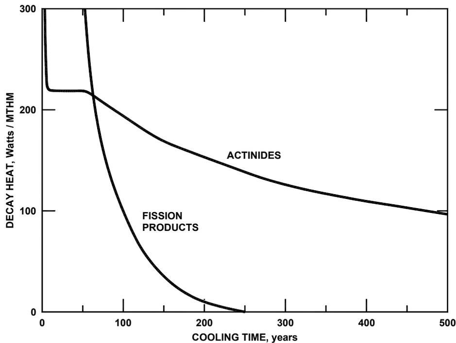
Figure 2. LWR spent fuel decay heat as a function of cooling time.
