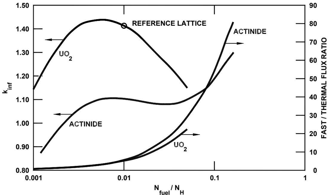
Figure 4. Spectral behavior of  $\text{UO}_2$  and actinide fueled LWR lattices.
